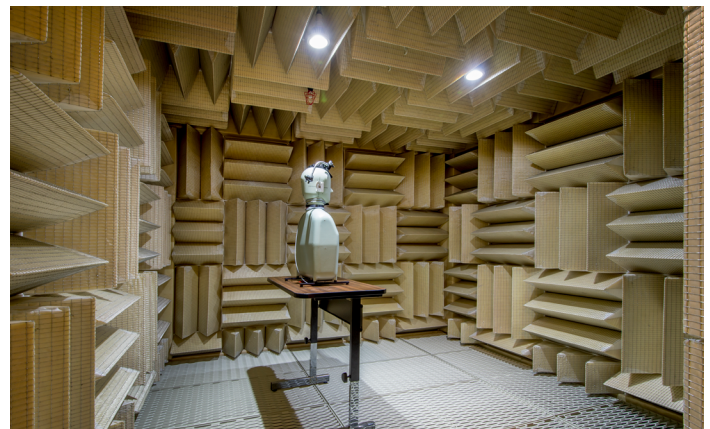
Anechoic (non-echoing) Chamber absorbs RF emissions for better measurements.
