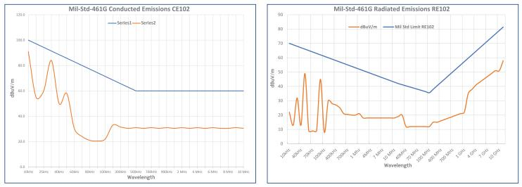
Conducted measurements are taken from the fixture power input leads in a laboratory. Radiated emissions are measured in an anechoic chamber designed to absorb indirect signals from the environment. The limits are shown in the red lines. Performance is shown on the yellow line. For more information on Mil-Std-461G see the Certolux Technical Brochure. Click here
