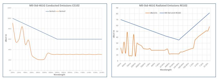
Conducted measurements are taken from the fixture power input leads in a laboratory. Radiated emissions are measured in an anechoic chamber designed to absorb indirect signals from the environment. The limits are shown in the red lines. Performance is shown on the yellow line. For more information on Mil-Std-461G see the Certolux Technical Brochure. Click here
