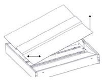
2. Carefully remove lens from luminaire by first sliding then lifting away from frame and place on clean surface top.
