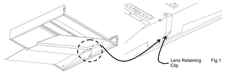
Tilt lens and insert above retaining clip(Fig.1) and to one end of fixture.
