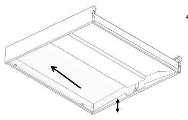
While holding lens in place on one end, raise the other end so that it clears the side flanges and gently drop lens to sit on interior flanges. Retaining clip may need to be re-pressed to allow lens to seat properly.
