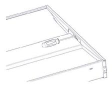
With flat screwdriver press gently retaining clip to release lens from frame
