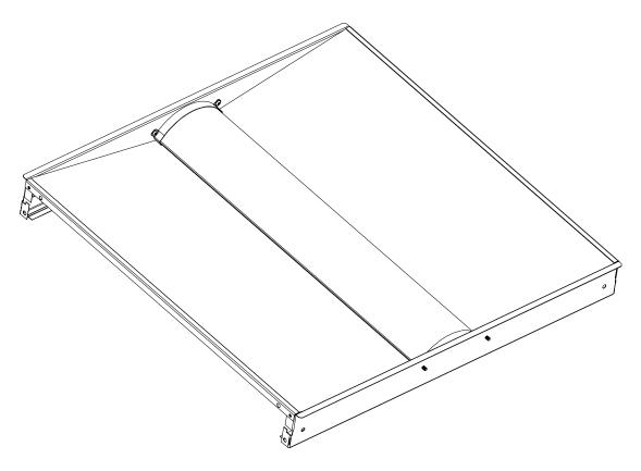
Diffuser retaining bracket comes with 2 tamper resistant center-pin Torx screws. For servicing luminaire from room side, a center-pin Torx screwdriver (by others) will be required to remove diffuser.
