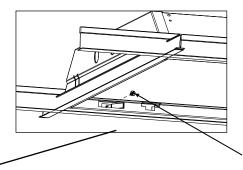
Self drilling screw, 1 at each end
