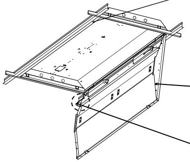
**Note:** Ensure safety tether cables are secured to fluorescent fixture prior to commencing with electrical connections.
