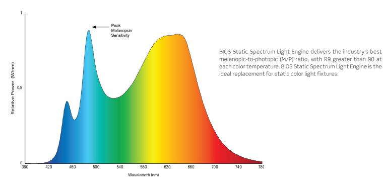
Static Engine Spectral Power Distribution (3500K)
