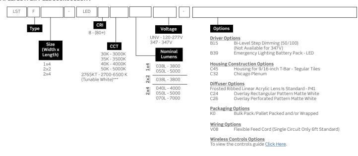
\*\*\* When Selecting 2765KT, if a tunable white-compatible control is not selected the luminaire will come standards with two sets of 0-10V wires for dimming and color tuning (see tunable white diagram for details). For compatible control options please consult factory Other options may be available, consult factory. Specifications and data
